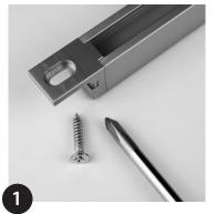
Select suitable screw for material to be installed. Prepare slot for recessing. Semi recessed minimum depth = 12mm Fully recessed minimum depth = 15mm
