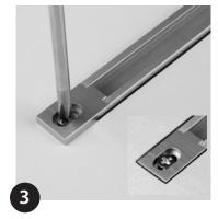
Can be installed semi-recessed as shown, fully recessed flush OR into specific s/steel handrail hardware - Consult with your handrail manufacturer/supplier before specification. For flush install L12mm Nylon spacer washers would be recommended under each end cap.
