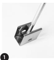
Fix clips with suitable screws. (min 3 clips per metre or every 500mm/20").
